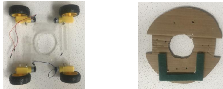
Figure 17: The 4-wheel driving version and hard-paper-base version
